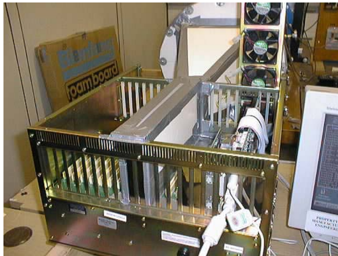
Figure 1. The test configuration shown is used for measuring airflow impedance for a “Sandwich” of Three PCBs, approximating airflow in an enclosure. Air is drawn through the PCBs through the transition section and into the air flow chamber at the rear.
